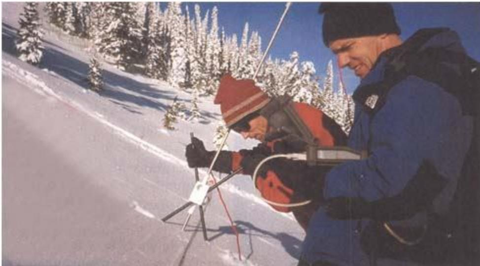
*A probe called the SnowMicroPen helps avalanche scientists detect weak layers of snow near the bottom of a snowpack.*
