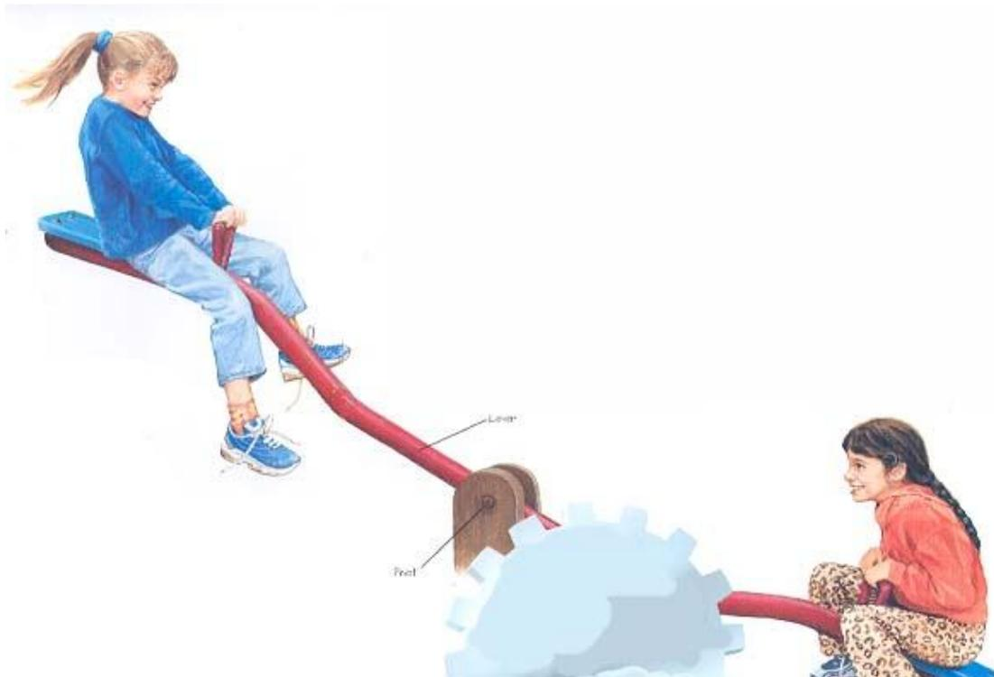
*On a seesaw lever, the pivot is in the middle. Other levers have pivots at the end.*
